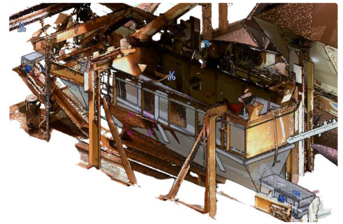
● CONVEYOR & HOPPER, REVERSE ENGINEERED
