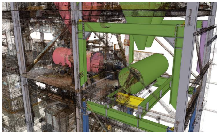
• NEW STEEL MODELLED INSIDE THE MEASURED CLOUD
